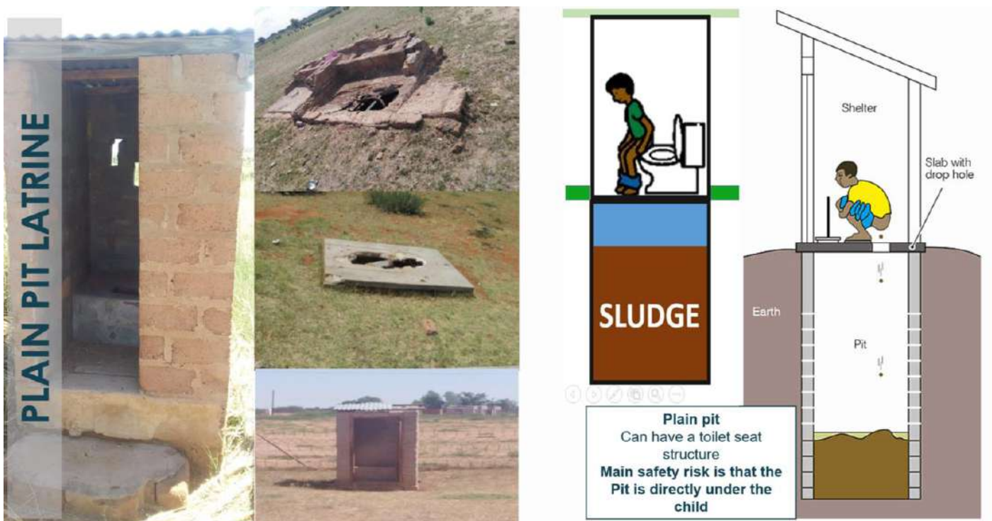
Figure 1: Explanation of PIT Latrines
